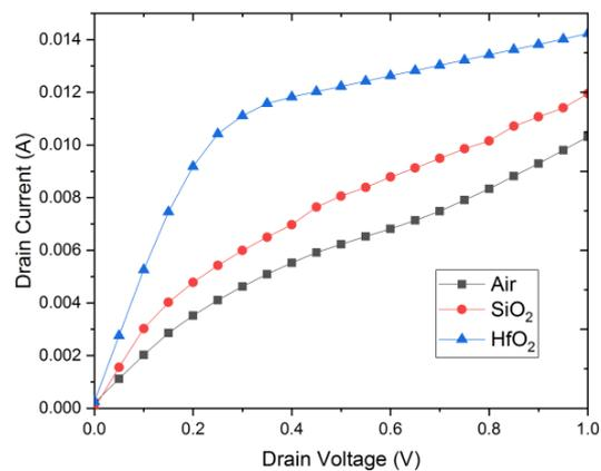
Fig. 5. I<sub>D</sub> VS V<sub>DS</sub> curves for different gate materials.
