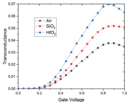
Fig. 10. Variation of  $g_m$  for various gate voltages.
