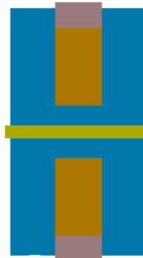
Fig. 4. Top view of proposed FinFET.
