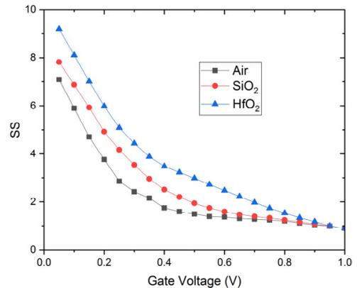
Fig. 9. Variation of SS for various gate voltages.
