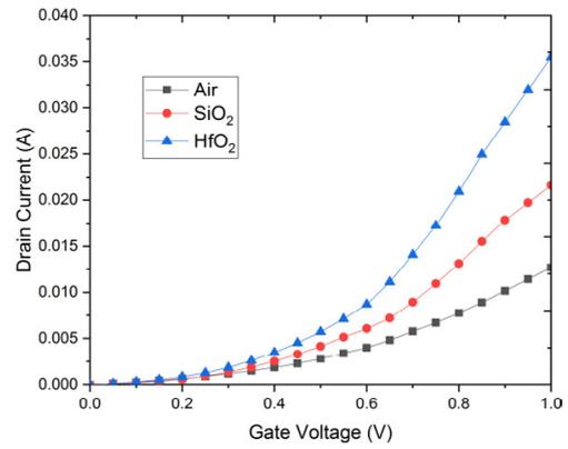
Fig. 7.  $I_D$  VS  $V_{GS}$  curves for different gate materials.
