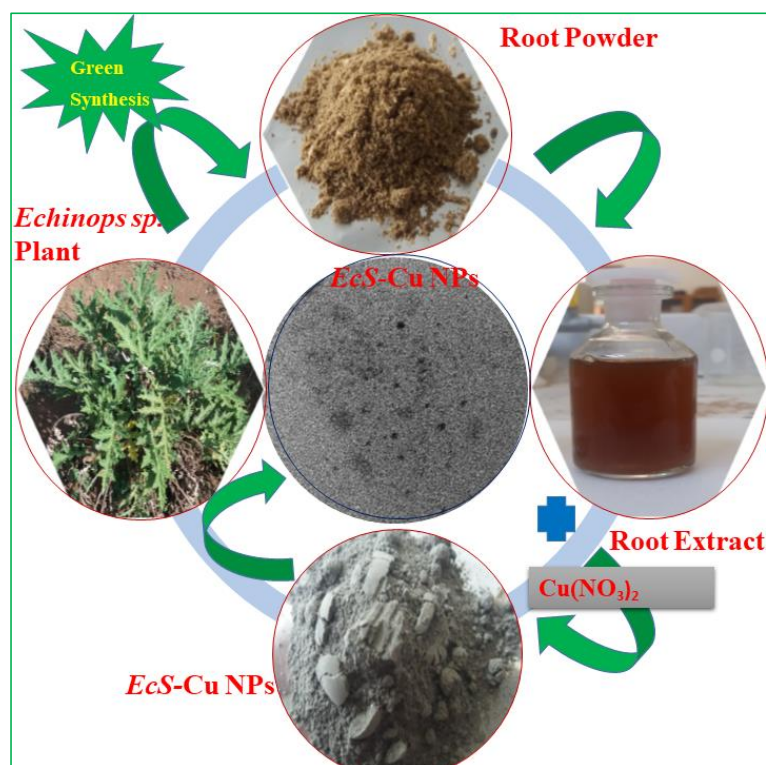
Fig. 1. The scheme of synthesis of EcS-Cu NPs .
