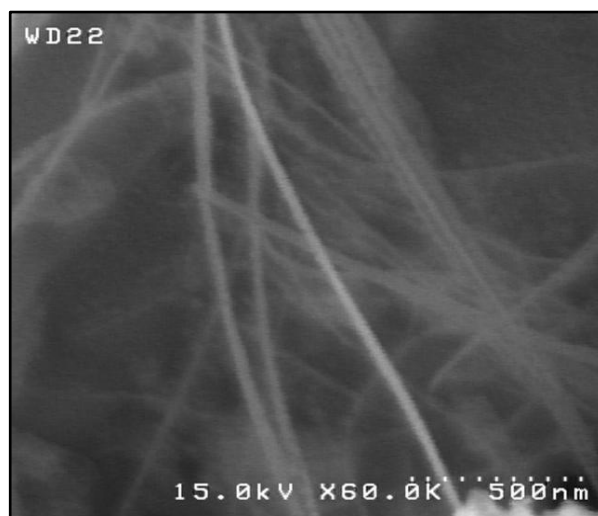
Fig. 2. SEM image of Mn_3O_4 nanowires.
