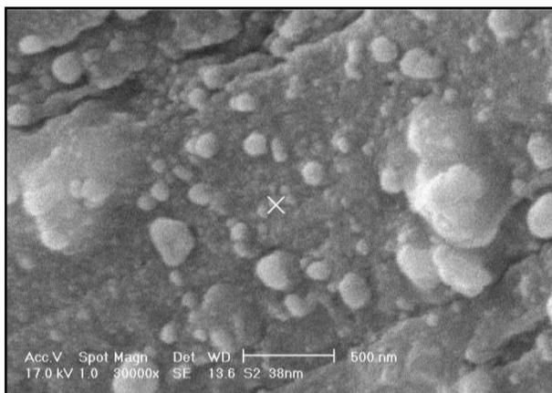
Fig. 1. Scanning Electron Microscopy(SEM) of Ag-PANI nanocomposite
