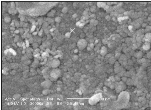
**Fig. 3.** Scanning Electron Microscopy (SEM) of Ag-PANI nanocomposite in concentration of 0.1 M  $\text{FeCl}_3$
