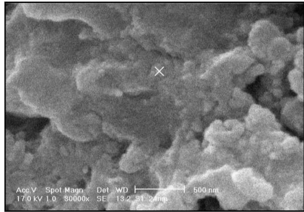
**Fig. 4.** Scanning Electron Microscopy (SEM) of Ag-PANI nanocomposite in concentration of 0.001 M silver nitrate
