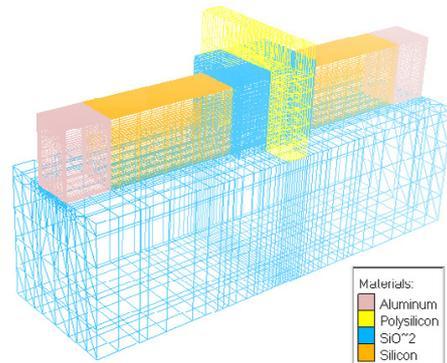
Fig. 3. 3D meshing view of proposed FinFET.
