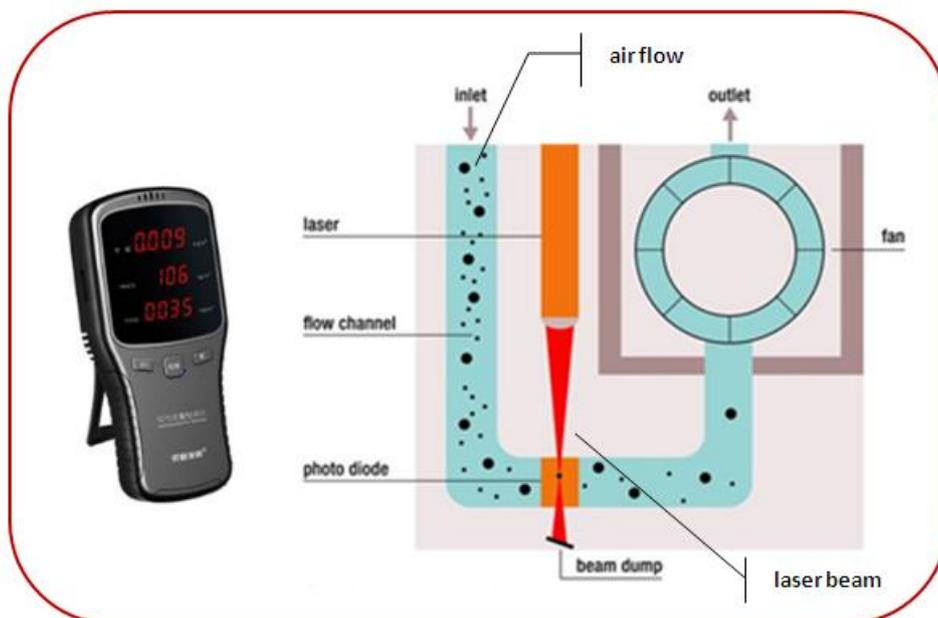
Fig. 2. Working principles of WP6910T indoor air quality monitor.
