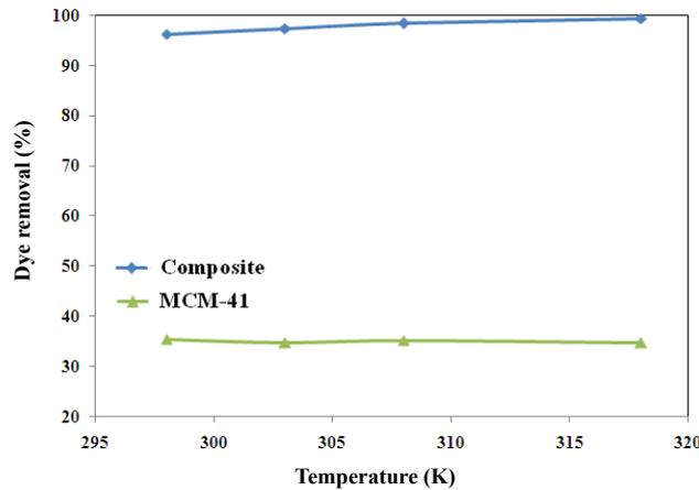
Fig. 8: Effect of temperature on dye removal percentage.
