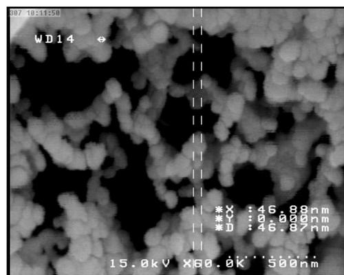
Fig. 2. The SEM image of cadmium(II) oxide nanoparticles prepared by calcination of nano-size compound 1.
