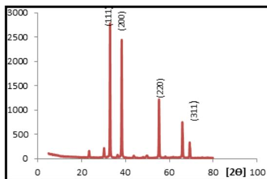
Fig. 3. XRD pattern of the prepared  $\text{CdO}$  nanoparticles
