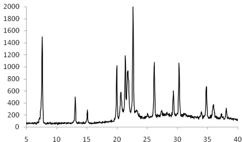
Fig.2. XRD pattern of the prepared  $\text{AlPO}_4\text{-5}$  crystals
