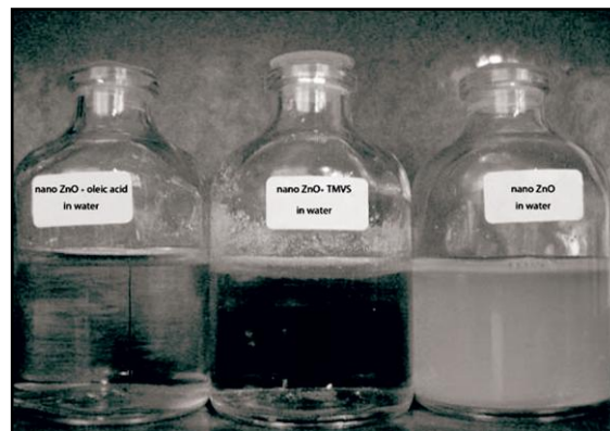
Fig. 1. ZnO nano-particles dispersed in water after 24 h under aerobic conditions. Modified with oleic acid (a), with TMVS (b) and unmodified ZnO nanoparticles (c).
