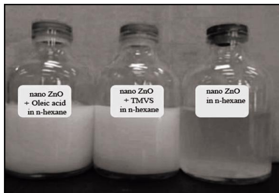
Fig. 5. ZnO nano-particles dispersed in n-hexane after 24 h under aerobic conditions. Modified with oleic acid (a), with TMVS (b) and unmodified ZnO nanoparticles (c).
