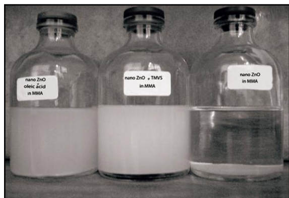
Fig. 4. ZnO nano-particles dispersed in Methylmethacrylate after 24 h under aerobic conditions. Modified with oleic acid (a), with TMVS (b) and unmodified ZnO nanoparticles (c).
