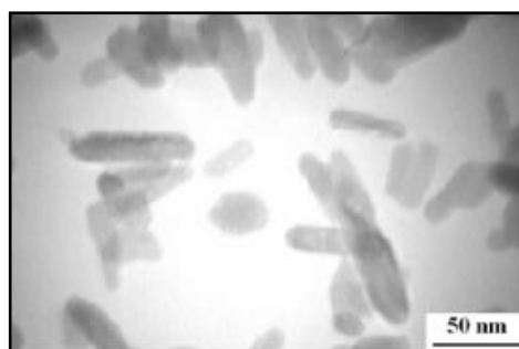
Fig. 3. SEM images of nano- fluorohydroxyapatite.
