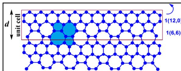
**Fig. 1.** Schematic representation of the carbon nanotubes junction composed one slice zigzag (12, 0) contacts to one slice armchair (6, 6) via the pentagon–heptagon pairs as topological defect in carbon hexagonal network. The rolling of the nanotube is indicated by arrow. The length of unit cell in the superlattice is  $d$ .
