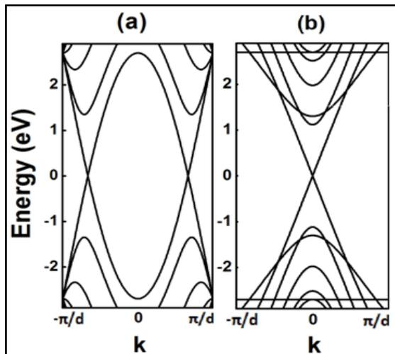
**Fig. 2.** The subband structures of single-walled (a) armchair tube (6,6) and (b) zigzag tube (12,0), which the lengths of unit cell are  $d=1.42 \text{ \AA}$  and  $d=4.26 \text{ \AA}$ , respectively. Fermi level is at zero energy.
