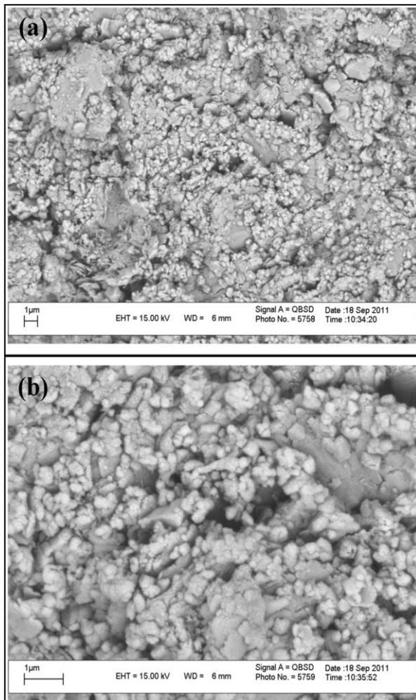
Fig. 3. Microstructure of normal concrete at different scale
