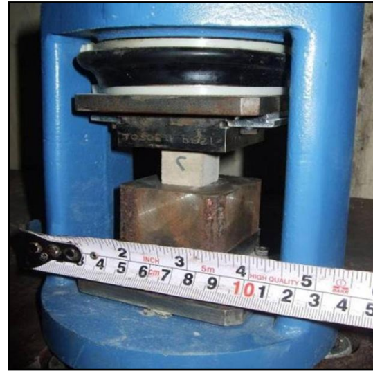
Fig. 4. Testing of the 20-mm paste cubes
