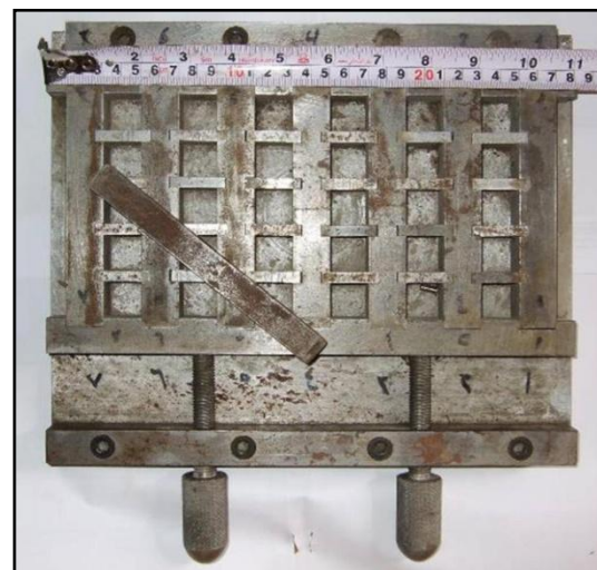
Fig. 3. Steel mold and tamper for casting the paste specimens
