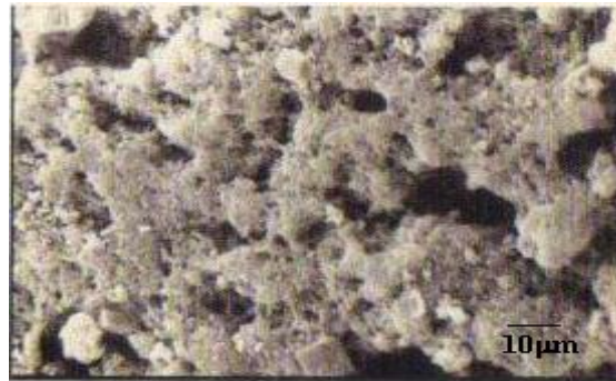
Fig. 2. SEM image of cobalt oxide dispersed PVA nanocomposite film.
