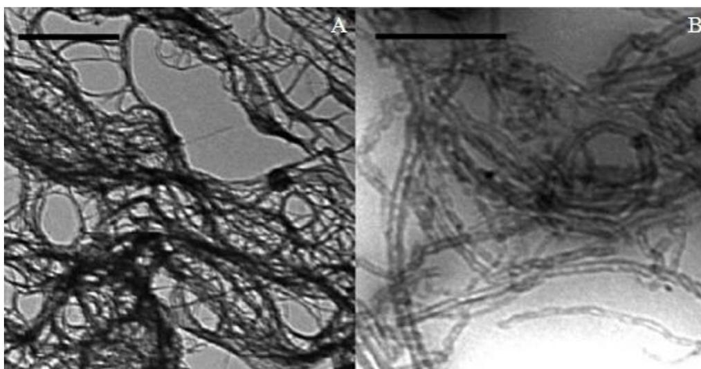
**Fig.2.** TEM images of single (A) and multi-walled (B) carbon nanotubes, While SWNT are present as bundles of different diameter and length, due to their strong aggregation tendency, MWNT can be instead observed as isolated entities. The scale bars correspond to 1  $\mu\text{m}$  and 250 nm, respectively
