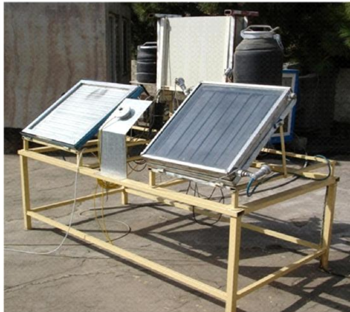
Fig. 3: The schematic of test loop and the experimental setup for DASC and FPSC outdoor performance test.
