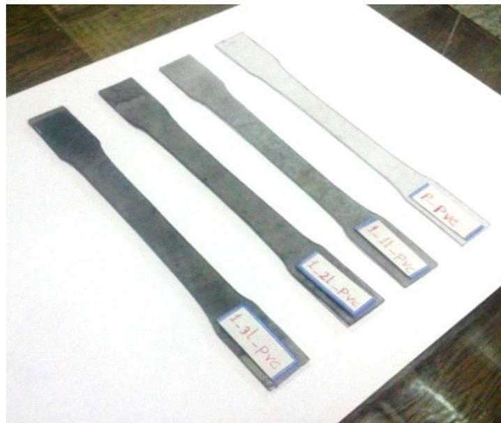
Fig. 2: Standard samples of the tensile testing.
