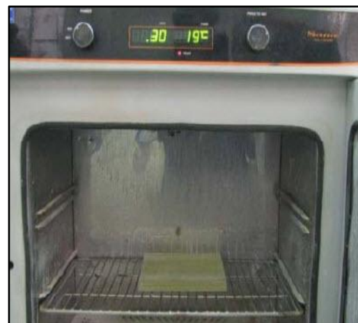
Fig. 4. Evaporation of ethanol from impregnated fibers.
