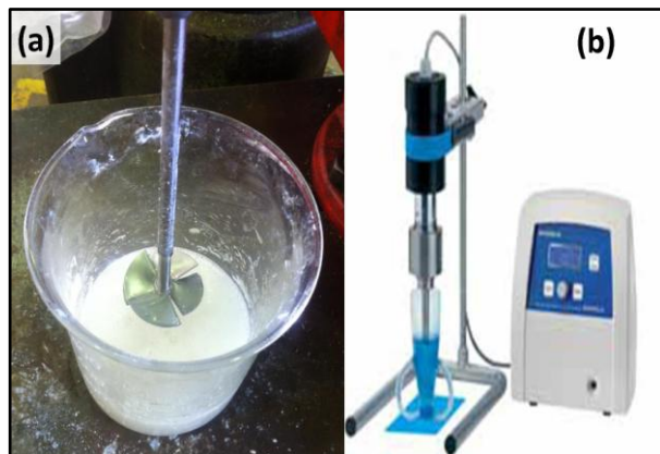
Fig. 2. Homogenizer (a) Mechanical blender; (b) Ultrasonic homogenizer.
