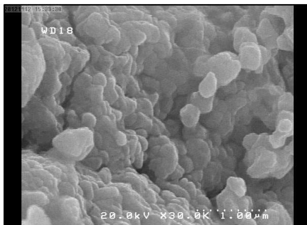
Fig. 5. SEM images of the \text{NiCl}_2 \cdot 6\text{H}_2\text{O} nanoparticles.
