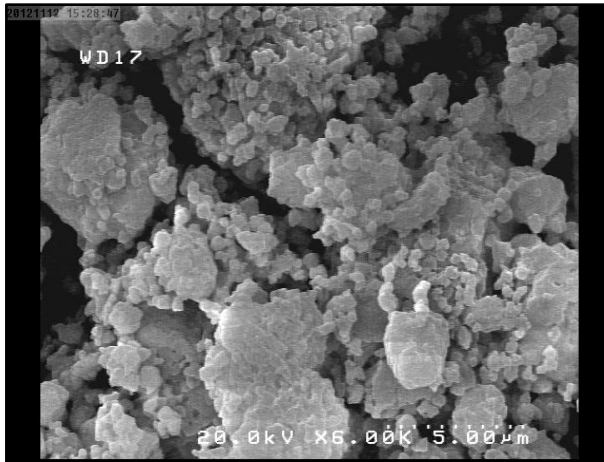
Fig. 4. SEM images of the \text{NiCl}_2 \cdot 6\text{H}_2\text{O} nanoparticles.
